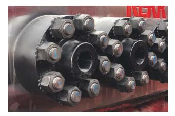
FIGURE 3. The F1X pump incorporates threaded hammer nuts and a bolt-on cover cap. (Source: Kerr Pumps)
