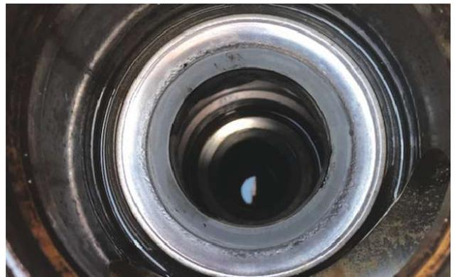
**FIGURE 2.** The use of tungsten carbide at the strike face of the Super Seat valve extends the operating life of the valve seat. (Source: Kerr Pumps)
