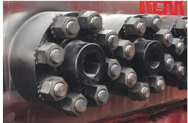
**FIGURE 3.** The FIX pump incorporates threaded hammer nuts and a bolt-on cover cap. (Source: Kerr Pumps)
